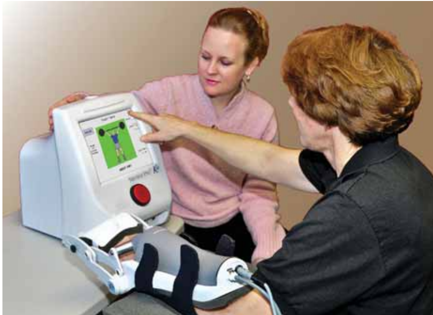
The Hand Mentor encourages the self-powered motion of the wrist and fingers and assists movement when necessary.
