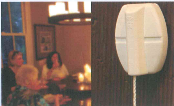
The pull cord, a component of a SimplyHome home-monitoring system, can be accessed to summon assistance, if needed.
